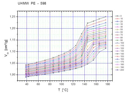
Fig. 2.1: Melting of UHMW PE, ITS runs [14Pio]
