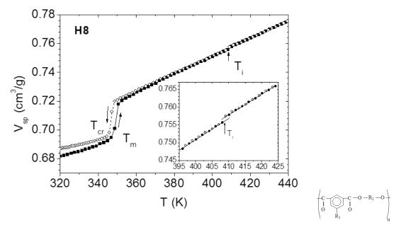
Fig. 2.3: Crystallisation and isotropisation of a semifluorinated polyester, IBA [02Got]
