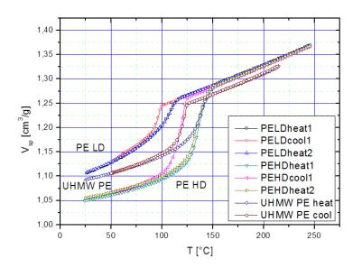
Fig. 2.2: Influence of chain branching on  $T_{\rm m}$  and  $V_{\rm sp}$  of different PE (IBA runs).
