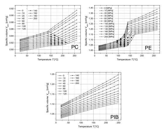
**Fig. 1.2:** Typical PVT behaviour of polymers showing glass transition (polycarbonate, PC Lexan 121), melting (poly(ethylene), PE-HD 25055E), or being in the liquid amorphous state in the whole measuring range (poly(isobutylene), PIB, laboratory grade). The open symbols characterise the stable quasi-equilibrium or equilibrium state of the polymers, the solid symbols the transition ranges. The regions are separated by lines to guide the eyes [own results].
