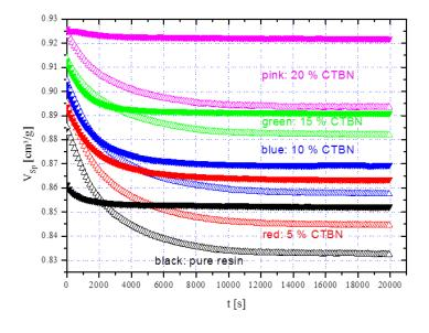
Fig. 2.5: Influence of rubber reactivity onto cure shrinkage of epoxy resin, DAQ run [07Mül]
