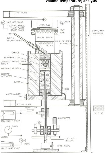
Fig. 1.1: Scheme of the GNOMIX PVT Apparatus
