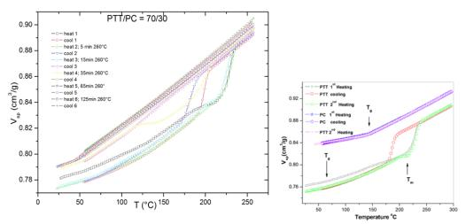
Fig. 2.6: Changes in glass transition, melting and crystallization, and specific volume due to transcrystallisation of PTT/PC blends, repeated IBA runs (the right images shows the behavior of the pure materials) [12Ara]
